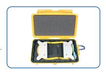
Portable Test Fiber Launch Box provides a calibrated span of optical fiber to evaluate near—end connectors and anomalies in network fiber systems. The Launch Box is placed between the system under test and an OTDR (Optical Time Domain Reflectometer) to improve the OTDR's ability to identify passive system components and abnormalities during system qualification and troubleshooting.
